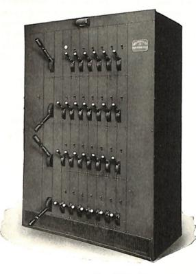
Our standard pre-set switchboards are of the dead front type and are built up in sections to meet the size requirements of various theatres, schools, colleges, lodges, and moving picture studios. A separate panel is provided for each branch circuit and one for each color master switch and dimmer handle. Each panel contains a double-pole, double-throw switch, the dimmer handle, if one is used, and a pilot lamp.
