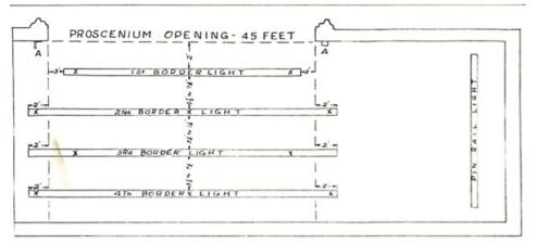
LIGHTING PLAN OF STAGE AT BORDER LIGHT HEIGHT A. Indicating Proscenium Lights. X. Indicating Working Lights in Border Lights.
