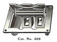
flush with the floor), provided with a hinged, self-closing cable notched door, so that it is always closed whether in use or not. A knockout is provided in the bottom of the box for one-inch conduit. These boxes are made in four sizes, namely, to hold one, two, three or four of our No. 690 receptacles and No. 688 plugs. These boxes are made to use on a two-wire circuit of any voltage up to 250 volts.
