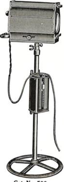
we recommend this spotlight equipped with spotlight dimmers. The spotlight consists of a small, neat, perfectly ventilated lamp house made of Wellsville Polished sheet iron with a cast aluminum front and back, mounted on a telescopic adjustable wrought-iron stand by means of a side bracket mounting or suspended in a yoke type mounting so that the hood can be raised, lowered, or tilted to any angle.
