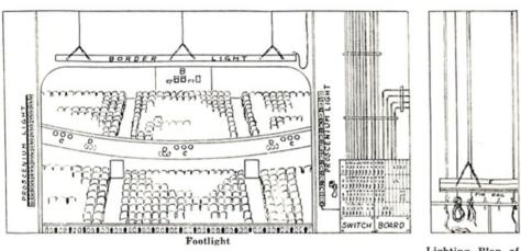
LIGHTING PLAN OF PROSCENIUM WALL, STAGE SIDE (Looking Out Into Auditorium) Lighting Plan of Stage Side Wall Showing Pin Rail and E Indicating Pin Rail Light.
